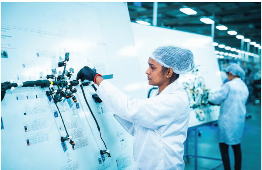
Assembly of a nail board as a physical guide for assemblers to assembly the wire harness.
